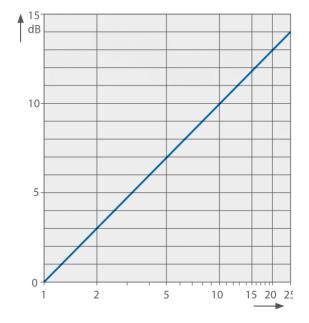
Fig. II: Addition of several sound sources
